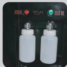
Oil injection & drain controlled by switch
